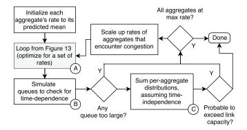
Figure 14: Iteration to assess statistical multiplexing.
