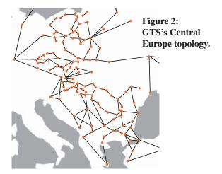
grid. An example of this class is GTS's network in central Europe, shown in Figure 2. Others, such as Cogent, span more than one continent, with good path diversity between continents. The long latency baseline between continents makes it easier to score well on latency stretch, but high LLPD also requires good connectivity within continents.
