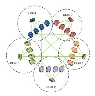
Fig. 3. DCell data center architecture.
