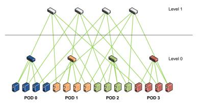
Fig. 4. BCube data center architecture.
