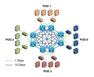
Fig. 1. Two-tier data center architecture.
