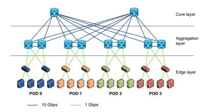
Fig. 2. Three-tier data center architecture.
