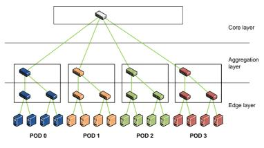
Fig. 6. Elastic-tree data center architecture.
