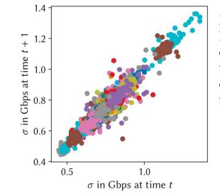
Figure 10: Minute to minute change of the standard deviation of traffic rate.
