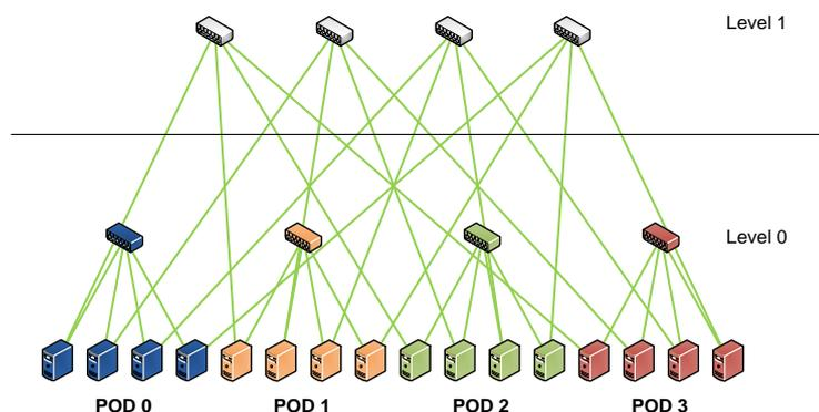
Fig. 4. BCube data center architecture.
