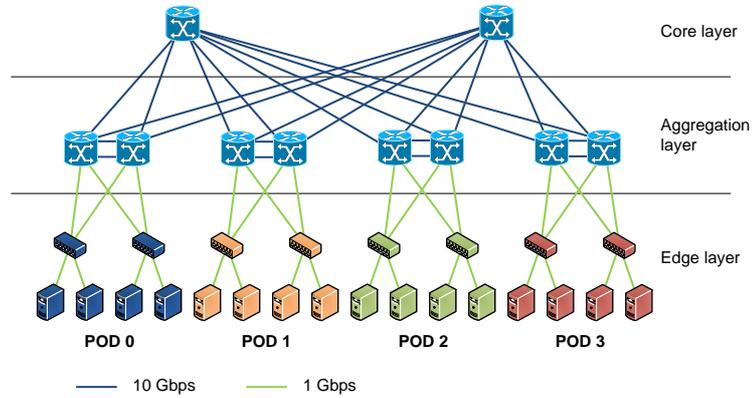
Fig. 2. Three-tier data center architecture.
