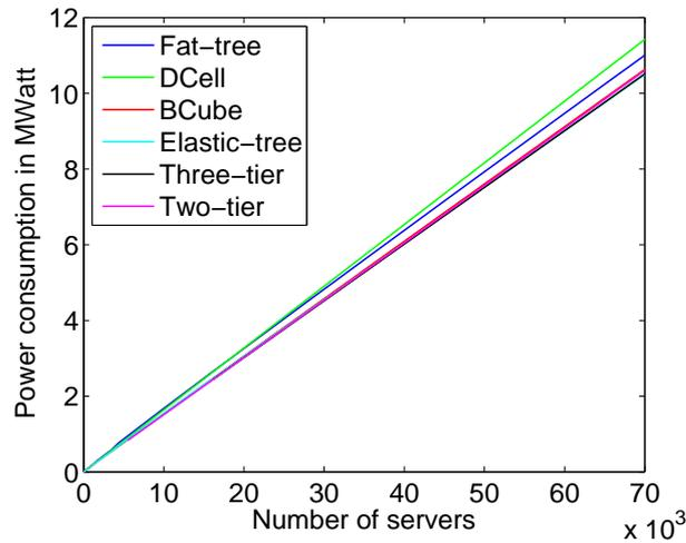
**Fig. 7.** Overall power consumption for different data center architectures.
